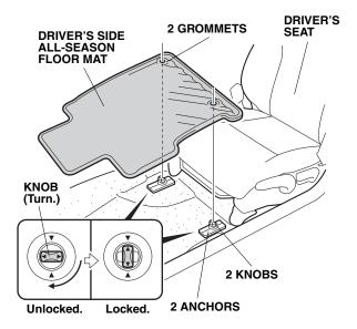
2. Place the grommets in the driver's side all-season floor mat over the anchors, and turn the knobs one guarter turn to secure the all-season floor mat.
